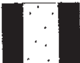
Appearance on the X-ray picture Sharp marked round blackenings
