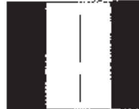
Appearance on the X-ray picture Dark continuous or interrupted line at the middle of the weld.
